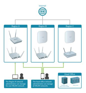
Through software-based monitoring and remote management of all wireless Access Points (APs) on your network, Nuclias Connect offers tremendous flexibility compared to traditional hardware-based unified management systems. Configuration can be done remotely. Network traffic analytics are available at a glance (in whole or in part). Load Balancing, Airtime Fairness, and Localized Throttling are enabled.
